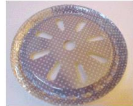
Inverted fused susceptor tray with vent slots
