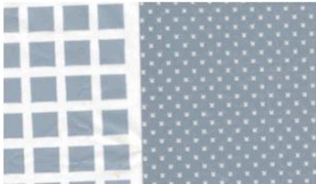
Patterned susceptor (left) and fused susceptor (right)
