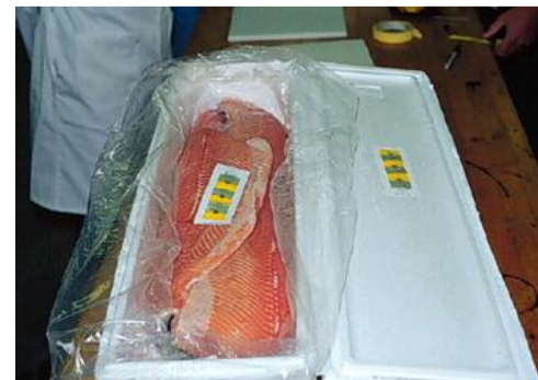
Activated VITSAB TTI's accompanying salmon fillets packaged with refrigerant destined for international airline freight
