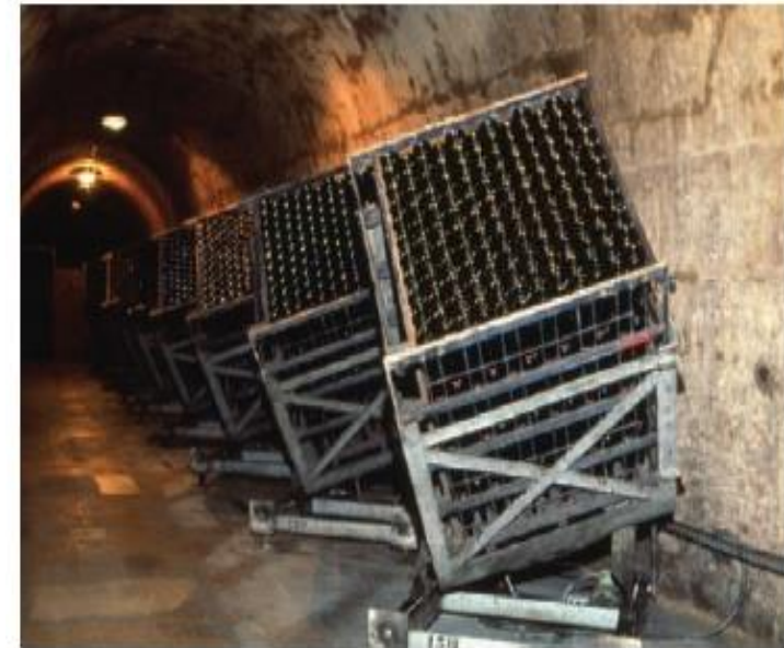
Plate 9.6 Mechanical riddling machine in Champagne. (Photo courtesy of Peper-Heidsieck, France)
