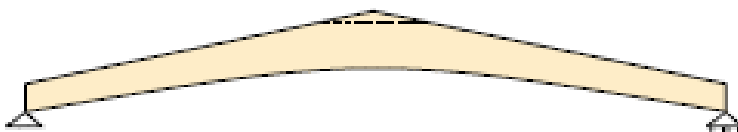
Bent ridge beam
