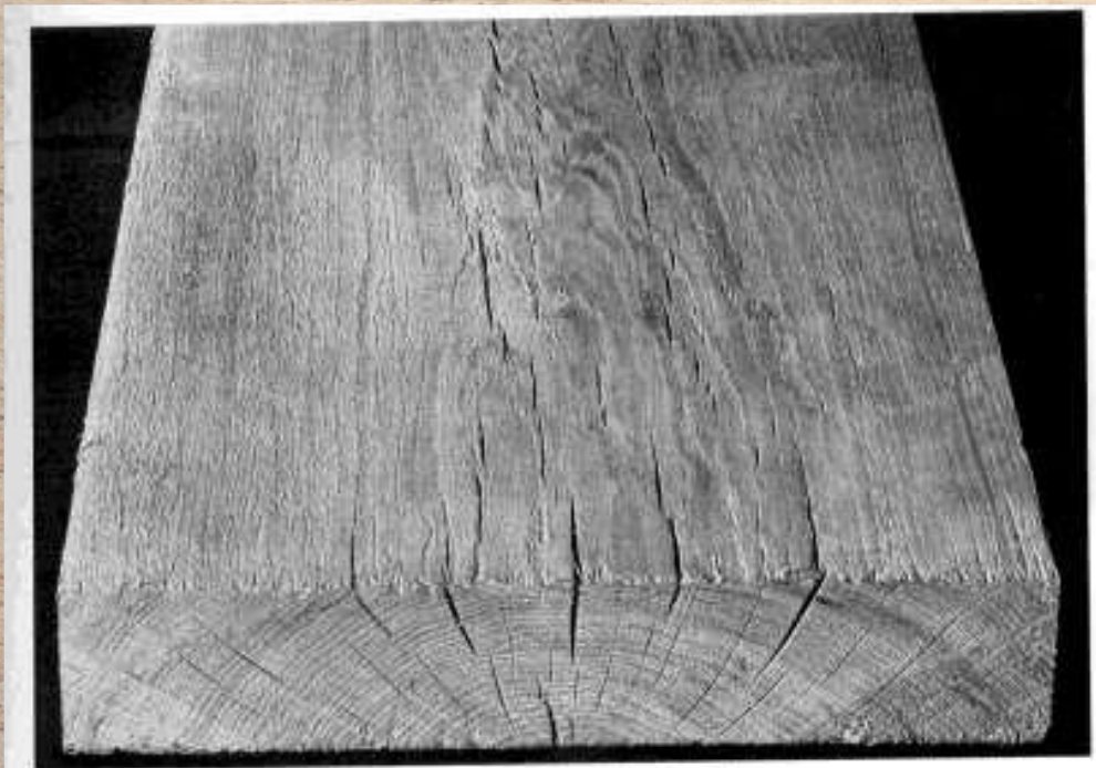
Plate 6: Plank of oak showing surface checking, end splitting and end checking
