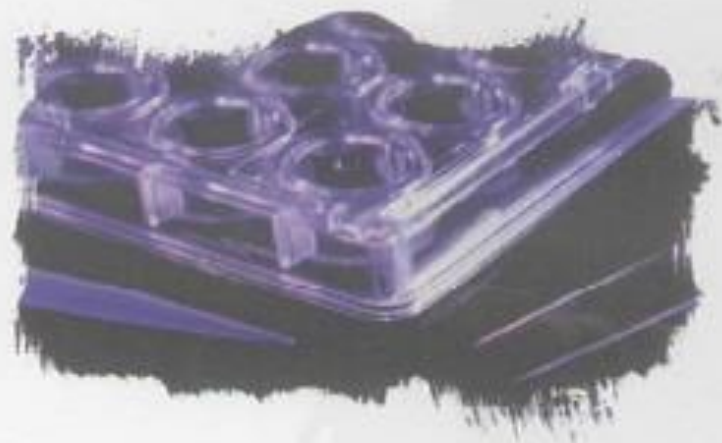
Figure 5.23. (A) Photograph of a vapor diffusion hanging-drop experiment over the well of a VDX plate. (B) A close-up of the hanging drop on the coverslip. (Courtesy of Hampton Research.)
