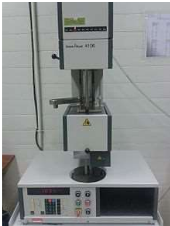
FIGURE Capillary rheometer (schematic).
